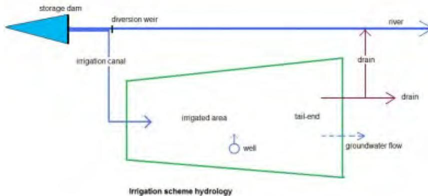
An irrigation scheme often draws water from the river and distributes it over the irrigated area. As a hydrological result, it is found that:
