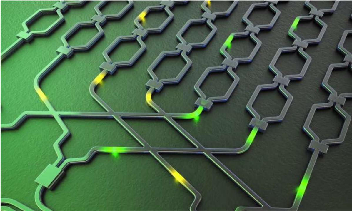
Tracks called waveguides guide photons in silicon, much like an optical fiber.
