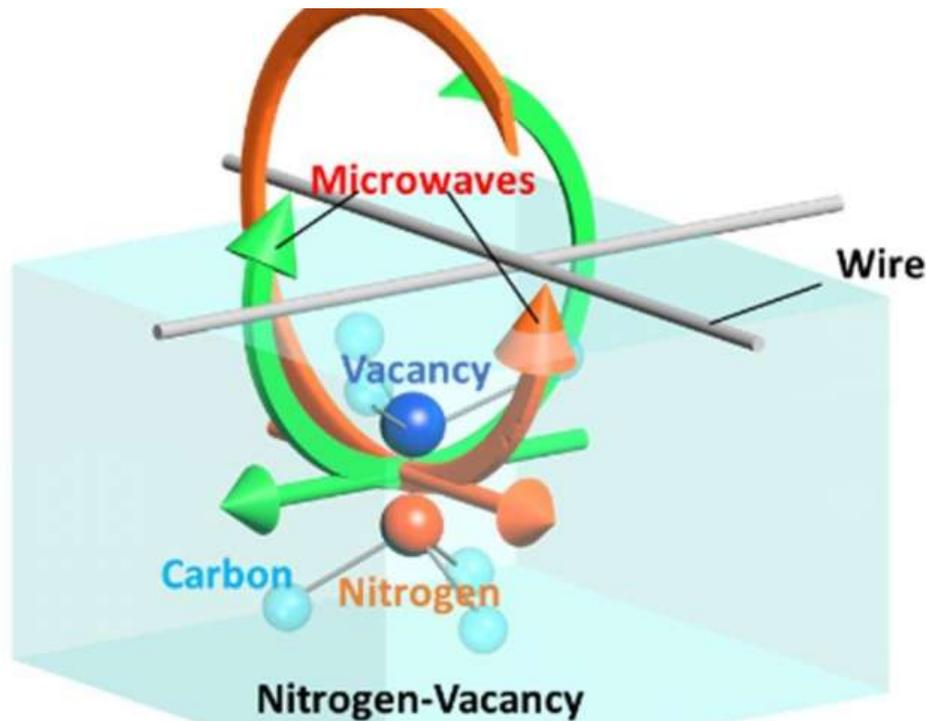
Nitrogen-vacancy (NV) center in diamond with two crossed wires for holonomic quantum gates over the geometric spin qubit with a polarized microwave. - Credit: Yokohama National University
